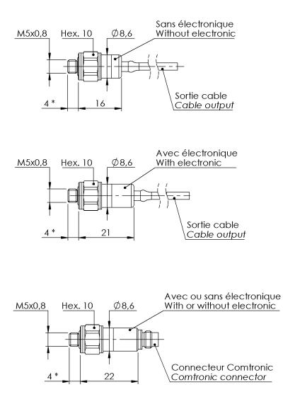
\* Option filetage allongé 10 mm 10 mm lengthened thread option
